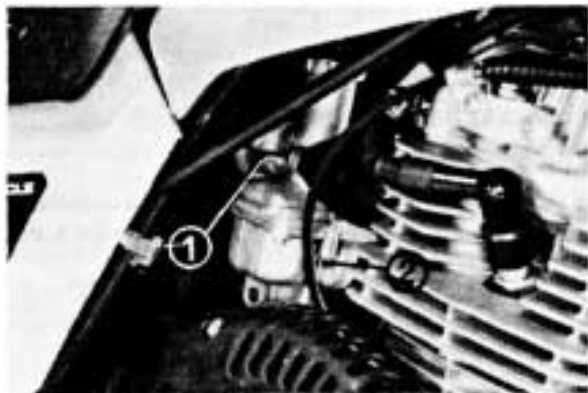
(1) Throttle stop screw (2) Pilot screw
