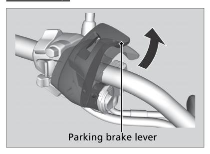
Place your motorcycle on a firm, level surface. Stop the engine and push your motorcycle while applying the parking brake lever to check the efficacy of the parking brake.
