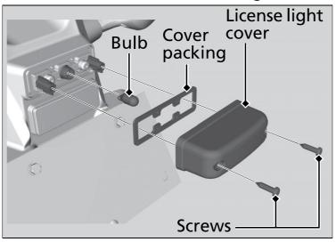
**3.** Install a new bulb and parts in the reverse order of removal.
