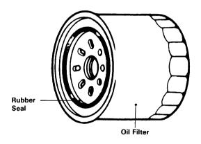
4. Install the new oil filter and tighten it: 10 N·m (1.0 kg-m, 7 ft-lb)
