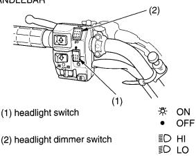
The headlight switch (1) is used to turn the headlight ON ( $^{*}$ ) or OFF ( $^{\bullet}$ ). To operate, turn the switch to ON ( $^{*}$ ) or OFF ( $^{\bullet}$ ).
