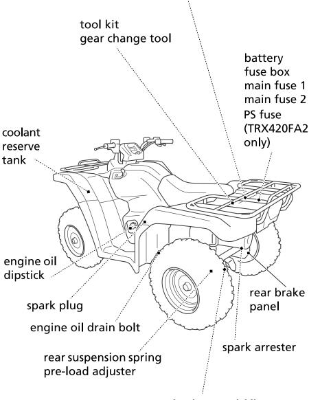
rear final gear oil fill cap rear final gear oil drain bolt
