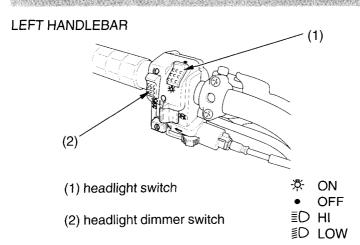
The headlight switch (1) is used to turn the headlights and assist headlight ON (%) or OFF ( $\bullet$ ). To operate, turn the switch to ON (%) or OFF ( $\bullet$ ).
