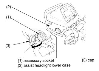
The accessory socket (1) is attached to the left side of the assist headlight lower case (2). You can use the accessory socket to power a trouble light, spotlight, CB radio, or cell phone, etc.
