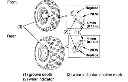
To check the condition of a tyre tread, measure the groove depth (1) in the centre of the tyre, or check the wear indicator (2).
