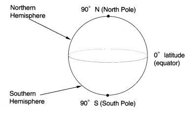
Each circle contains 360° (degree) Each degree contains 60' (minutes) Each minute contains 60'' (seconds)
