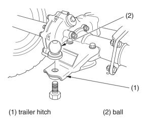
The trailer hitch (1) is located on the rear axle housing. To use the hitch, you'll need a proper size ball (2) as specified by the trailer manufacturer.
