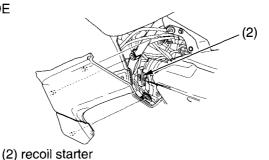
The recoil starter (2) is used to start the engine when the battery is low. See *Using the Recoil Starter*, page 67.
