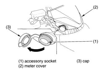
The accessory socket (1) is attached to the right side of the meter cover (2). You can use the accessory socket to power a trouble light, spotlight, CB radio, or cell phone, etc.
