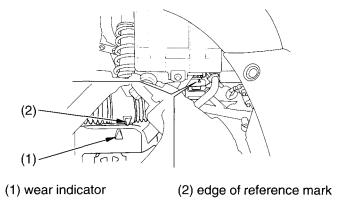
Check the wear indicator. If the wear indicator (1) aligns with the reference mark (2), replace both pads as a set, see your Honda dealer for this service.
