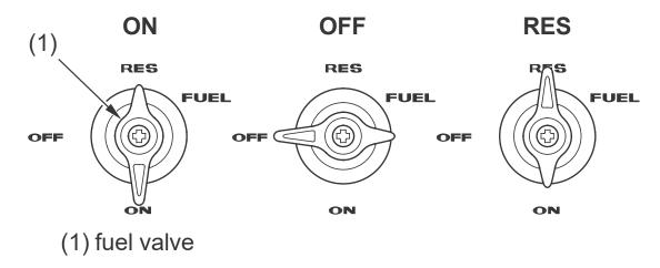
The manual fuel valve (1) is located on the left side under the fuel tank.
