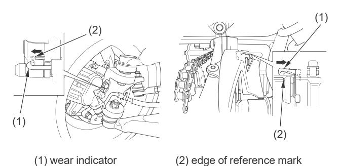
Front brake pads/Rear brake pads: If the wear indicator (1) aligns with the edge of the reference mark (2), both pads must be replaced, see your Honda dealer for this replacement.
