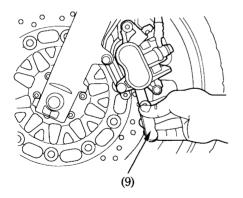
If the feeler gauge cannot be inserted easily, pull the left fork outward or push inward until the gauge can be inserted and tighten the axle pinch bolts with the gauge inserted. After tightening, remove the gauge. After installing the wheel, apply the brakes several times, then recheck both discs for caliper holder to disc clearance. Do not operate the motorcycle without adequate clearance.
