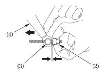
(2) Rear brake adjusting nut(3) Brake arm pin(4) Brake arm
