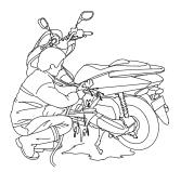
6. Test the brakes before riding the scooter. Several applications may be necessary to restore normal braking performance.
