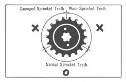
4. If the drive chain or sprockets are excessively worn or damaged, they should be replaced. Never use a new chain with worn sprockets; rapid chain wear will result.
