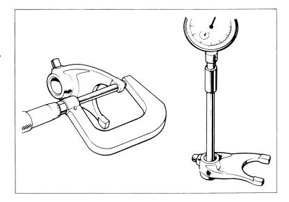
Check the shift fork shaft for wear, damage or bending.
