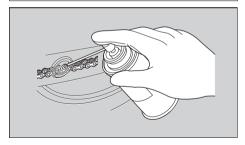
Never use gasoline or low flash point solvents for cleaning the drive chain.
