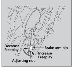
Apply the brake several times and check for free wheel rotation after the brake pedal is released. **3.** Push the brake arm to confirm that there is a gap between the rear brake adjusting nut and brake arm pin.
