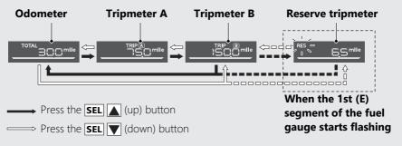
When the 1st (E) segment of the fuel gauge starts flashing, the odometer and tripmeters switches to the reserve tripmeter.
