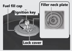
Do not fill with fuel above the filler neck plate. **Fuel type:** Unleaded gasoline only **Recommended fuel octane number:** Pump Octane Number (PON) 86 or higher
