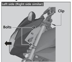
1. Remove the bolts and clip (▶ P. 54) on both sides and pull the headlight assembly forward.
