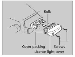
**3.** Install a new bulb and reinstall the parts in the reverse order of removal.
