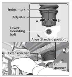
Attempting to adjust directly from 1 to 9 or 9 to 1 may damage the shock absorber.
