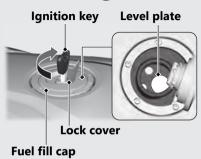
Do not fill with fuel above the level plate. **Fuel type:** Unleaded gasoline only **Recommended fuel octane number:** Pump Octane Number (PON) 86 or higher. **Tank capacity:** 4.62 US gal (17.5 L)
