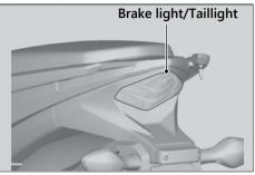
The brake light and taillight uses several LEDs.
