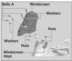
**1.** Remove the windscreen by removing the bolts A, washers and nuts.
