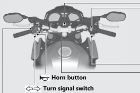
Pressing the switch turns the turn signal off.
