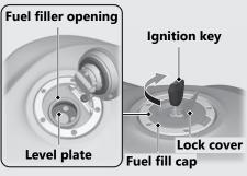
Do not fill with fuel above the level plate. **Fuel type:** Unleaded gasoline only **Recommended fuel octane number:** Pump Octane Number (PON) 86 or higher. **Tank capacity:** 4.57 US gal (17.3 L)
