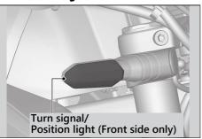
Each right and left front turn signal/position light uses several LEDs.
