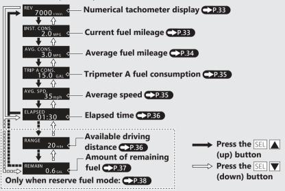
When the low fuel indicator lights and the low fuel pop-up information appear, INFO 3 display will automatically switches to the amount of remaining fuel display.
