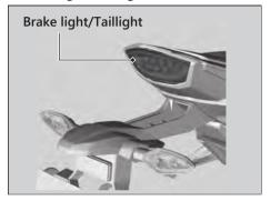
The brake light and taillight uses several LEDs.
