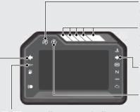
**Low oil pressure indicator** Comes on when the ignition switch is turned to the ON position. Goes off when the engine starts.
