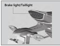
The brake light and taillight uses several LEDs.
