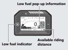
After refueling more than the reserve amount, the display returns to normal when the ignition switch has been ON position for about a minute.
