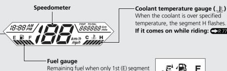
When the coolant is over specified temperature, the segment H flashes.
