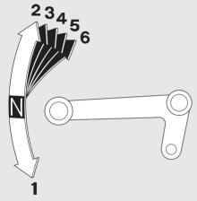
If you put the motorcycle in gear with the side stand down, the engine will shut off.
