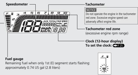
If the fuel gauge indicators repeat flashing or turned off: P.90
