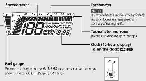
If the fuel gauge indicators repeat flashing or turned off: P.93
