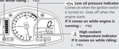
C PGM-FI (Programmed Fuel Injection) malfunction indicator lamp (MIL)
