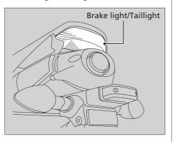
The brake light and taillight uses several LEDs.
