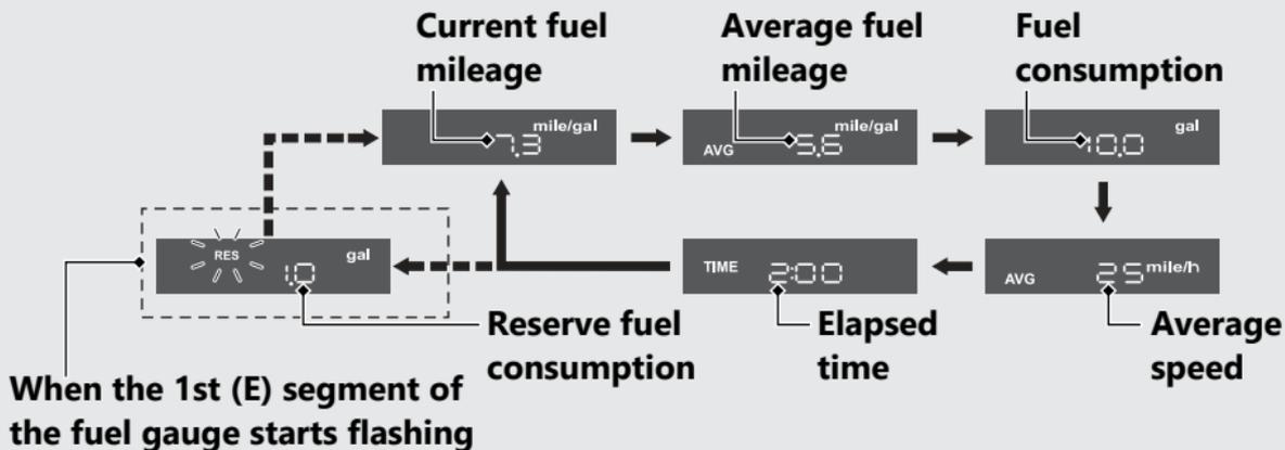
When the 1st (E) segment of the fuel gauge starts flashing, the current fuel mileage, average fuel mileage, fuel consumption, average speed or elapsed time switches to the reserve fuel consumption.
