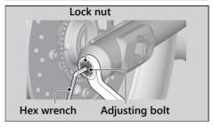
8. Tighten the rear axle nut.
