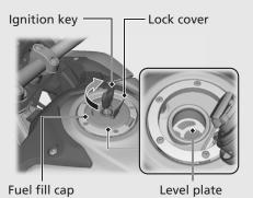
Do not fill with fuel above the level plate.
