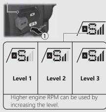
The selected level is maintained even when the ignition switch is turned to the OFF position, or transmission is switched to out of \$ mode
