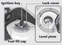
Do not fill with fuel above the level plate. Fuel type: Unleaded gasoline only Recommended fuel octane number: Pump Octane Number (PON) 86 or higher.
